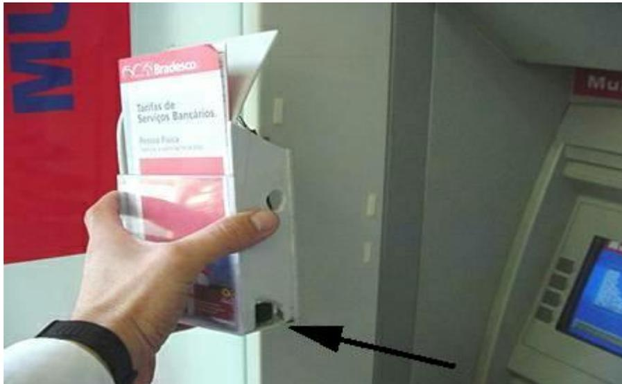
The PIN reading camera being installed on the ATM is housed in an innocent looking leaflet enclosure.
